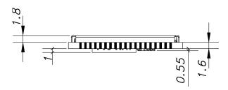
**Note** The NAND flash on the bottom of the ConnectCore 6UL module adds 1mm to the overall PCB thickness and is the tallest component on this side of the printed circuit assembly.
