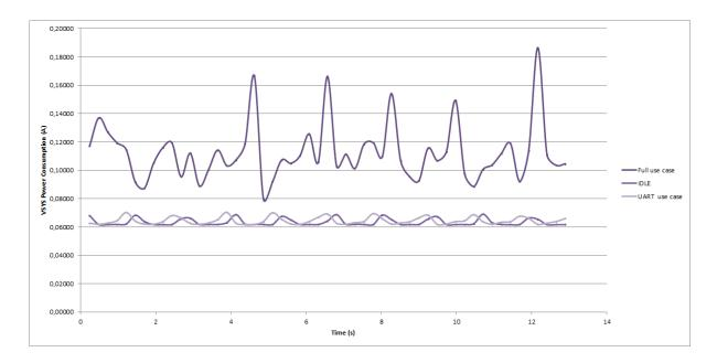
**Note** Average power consumption was calculated after approximately a minute of sampling data, but the plot shows power consumption over 13 seconds for a more detailed view of power consumption oscillations.
