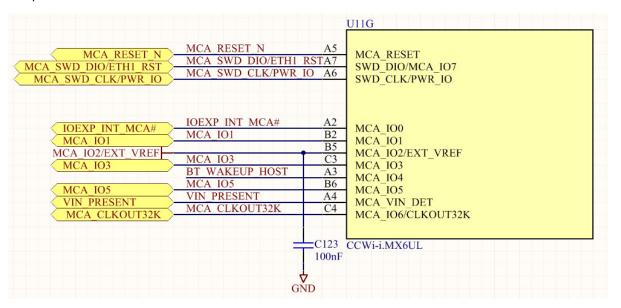
Note that the voltage reference continues normal operation in low power modes (suspend and power off). Therefore, if the voltage reference is enabled during normal operation but is not required for low power operation, Digi recommends using the software to disable it before entering low power in order to minimize the power consumption, and re-enable it when resuming normal operation.
