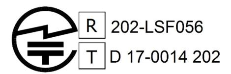
**Note** Due to space constraints, the ConnectCore 6UL module label doesn't support radio marking for Japan. If space allows, end product label should support radio marking for Japan. If not, radio marking shall be documented in the user manual.
