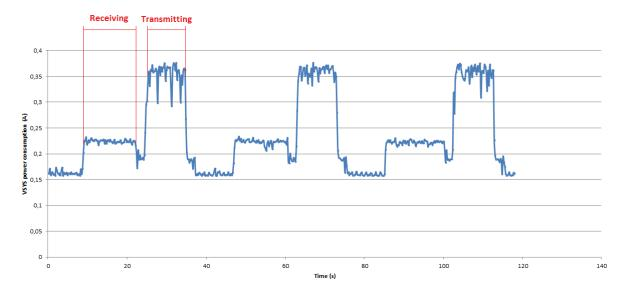
The power consumption increase of the real wireless transmission is calculated by taking the mean power consumption value of the transmission and receiver bursts:
