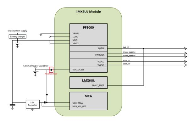
Digi has validated this hardware configuration with the Panasonic DB2J31400L diode. It's low reverse leakage current (300 nA) is ideal for this low-power mode application.
