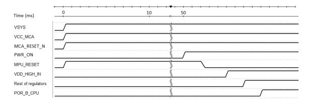
To optimize the power-up sequence, Digi suggest a configuration that controls the main input power supply of the SOM (VSYS) through the PWR\_ON line (e.g. through a power switch). For more information, see the detailed hardware implementation in the ConnectCore 6UL SBC Pro reference design schematics. In this case, VSYS won't be enabled until the MCA drives the PWR\_ON line high. The following simplified time diagram illustrates this particular case:
